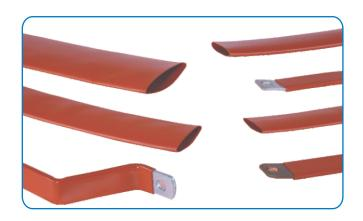
Bus Tube is heat shrinkable tube designed to insulate busbar systems up to 66KV & to protect against accidental flash-over. The tubes are manufactured from high quality non tracking crosslinked polyolefin material. Meets ANSI C37.20.2 standards for switchgear application up to 66 kV.
