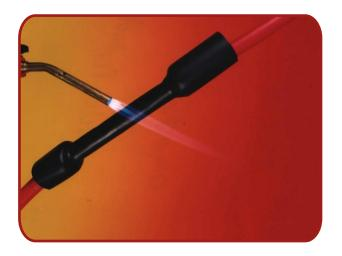
GDW is dual wall tubing manufactured by co-extrusion of polyolefin and hot melt adhesive. Designed to provide both insulation and sealing for protected articles.
