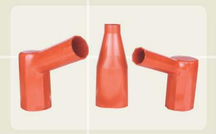
Angleboots are Heat Shrink Right Angle / Straight Boots, which provides insulation to the bushings in the cable termination box, where the clearance between phase to phase and phase to earth is less then the normal air clearance. These boots provide protection against flash-over in the event of high humidity, rodent menace and surge impulse.
