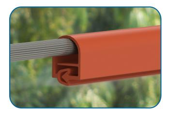
Insulcover is a Wrap Around Line Cover that provides retrofit insulation for Overhead Conductors to help prevent electrical outages caused by trees or wildlife coming into the contact with distribution lines. It is manufactured from high quality Non-tracking Cross-linked Polyolefin material. Gala Overhead Line Covers can be used in many applications upto 66 kV.
