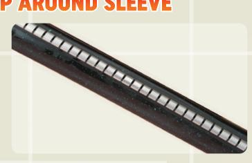
Insulsleeve is a Cross-linked polyolefin 'tube' which is folded around the cable/pipe, zipped up with a stainless steel channel and then heat shrunk.
