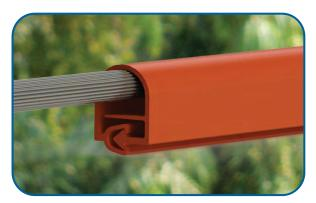
Insulcover is a Wrap Around Line Cover that provides retrofit insulation for Overhead Conductors to help prevent electrical outages caused by trees or wildlife coming into the contact with distribution lines. It is manufactured from high quality Non-tracking Cross-linked Polyolefin material. Gala Overhead Line Covers can be used in many applications to enhance the insulation up to 400 kV.
